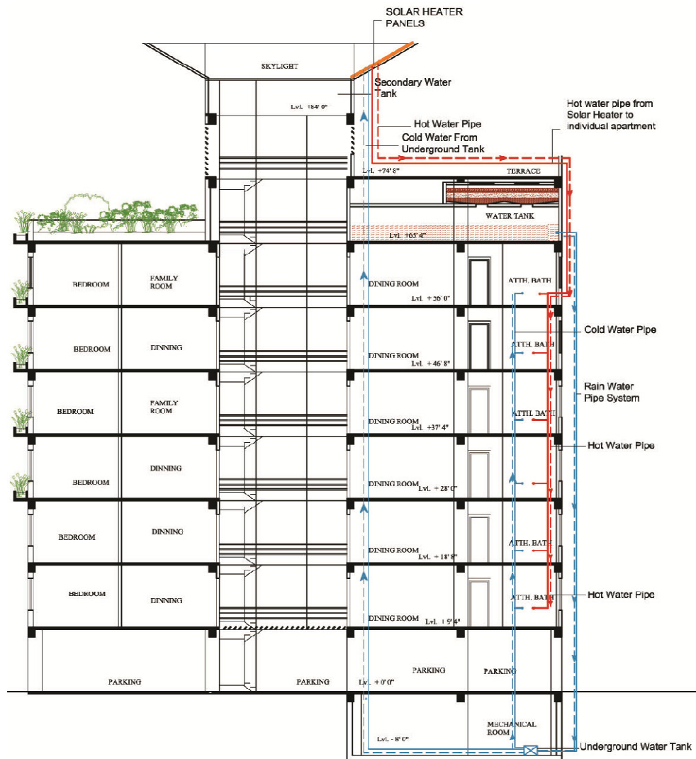
Figure 9.15 - Solar water heating system
